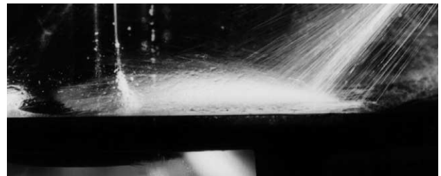
Fig. 5. Spray rebound from manifold floor: injector block 1; valve head diameter D_V = 25 mm.
