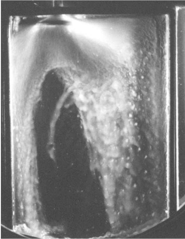
Fig. 13. Fuel distribution showing the flow patterns on the side walls ( z = 15 mm).
